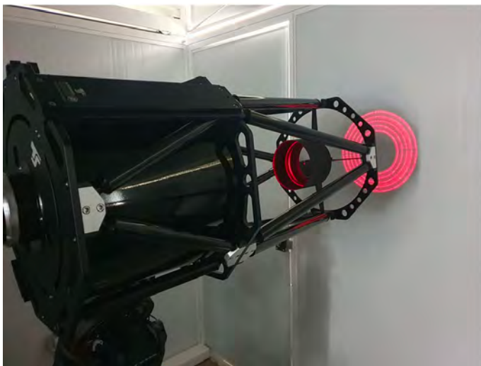
Figure 3 — Laser-ring collimation of the Ritchey-Chrétien telescope, showing the alignment pattern before and after adjustment.
