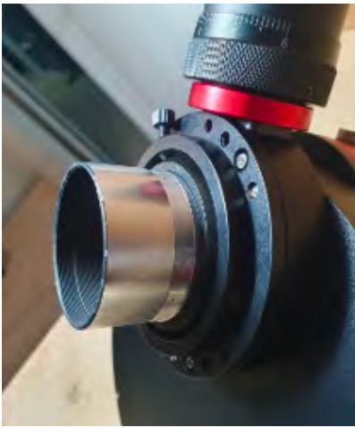
Figure 6 — Camera adapter coupling where a loose screw caused micro-vibrations and uncorrectable guiding drift.
