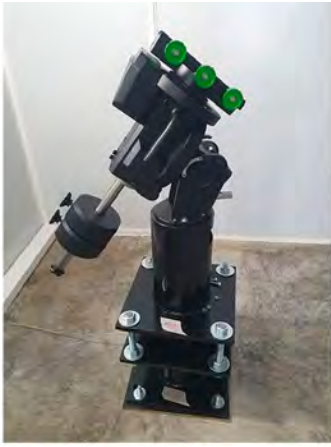
Mount Installation on a Custom Permanent Pier
