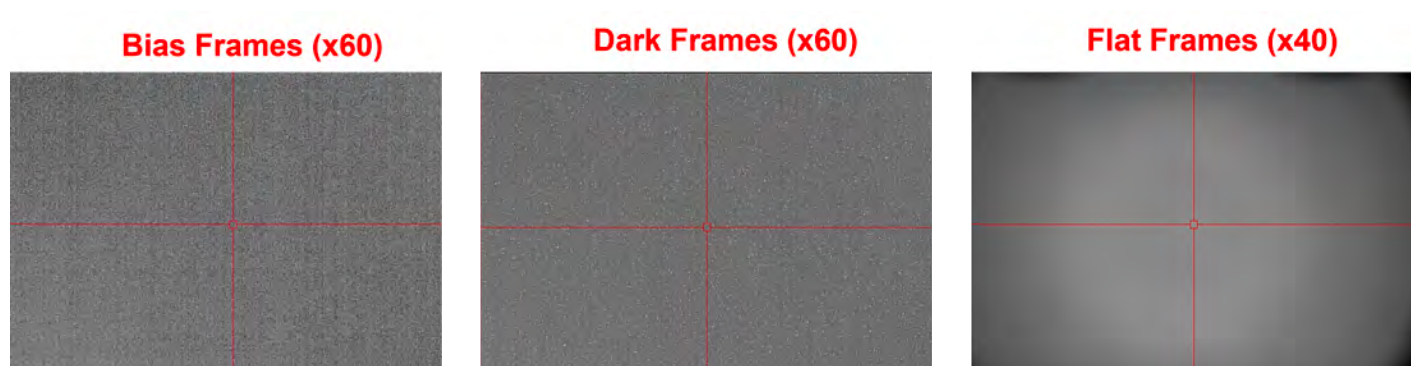
Figure 5 — Example bias, dark, and flat calibration frames used to remove camera and optical systematics from science images.
