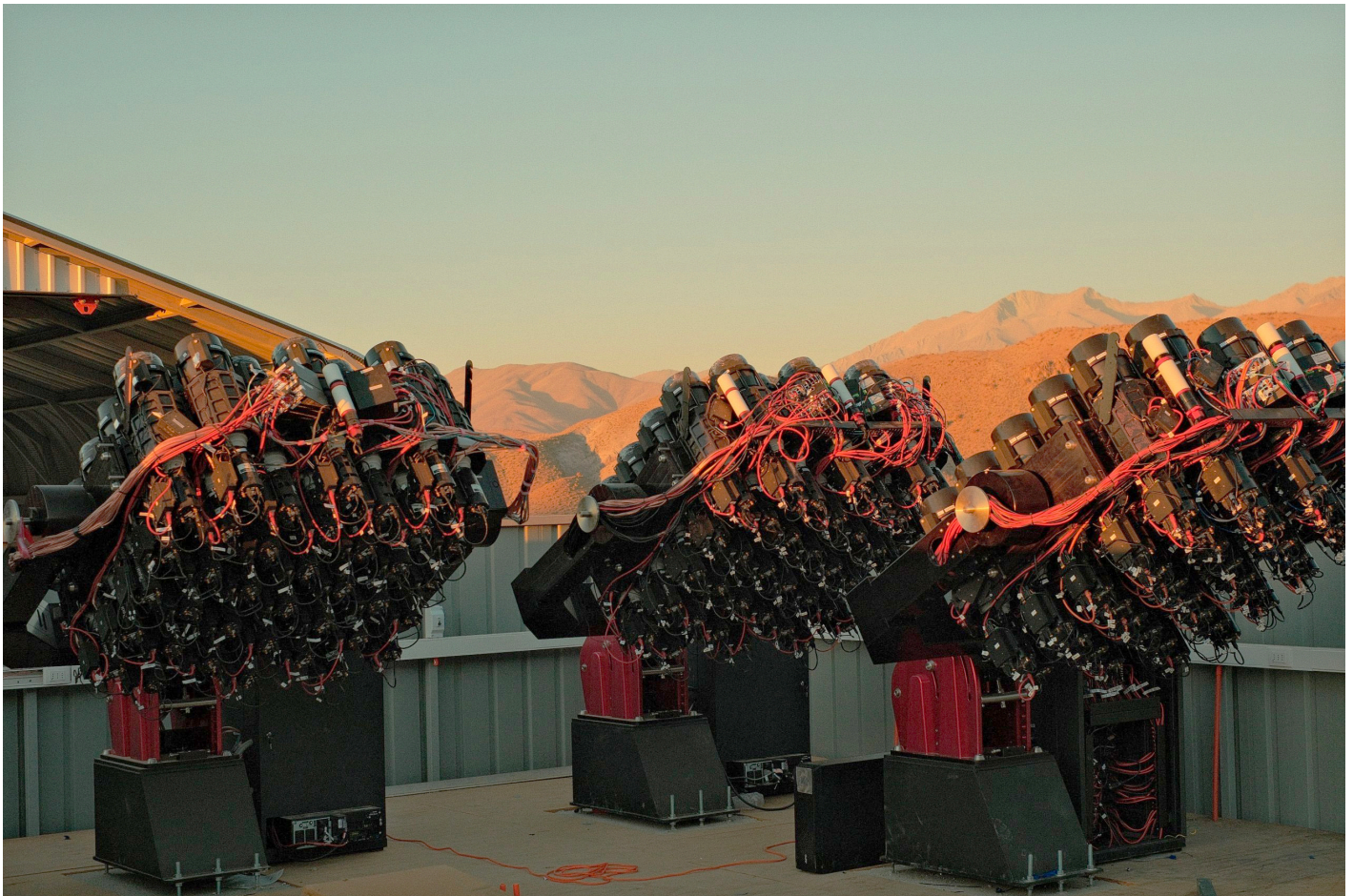
Figure 2 – A rendering of part of the MOTHRA telescope. Each of the mounts has 38 high end Canon telephoto lenses, equipped with special filters to observe the cosmic web. The completed telescope will have 30 mounts, in two buildings, with a total of 1,140 lenses. Credit: Dragonfly FRO.
