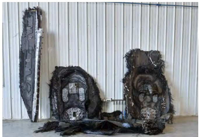
Figure 1 — Pieces of a SpaceX Crew Dragon Cargo Trunk that fell on farmland near Ituna, Saskatchewan, in 2024. Barn cat on the far right for scale. Photo taken by the author.
