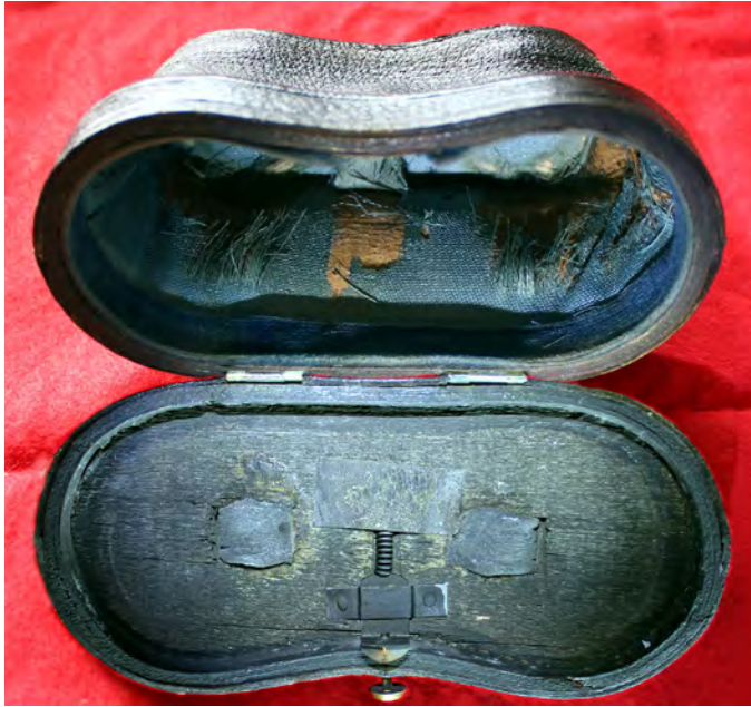
Figure 14 — Interior of the case for the Potter field glasses showing the satin lining, and wooden form and closure of the lid. Photograph by R.A. Rosenfeld.
