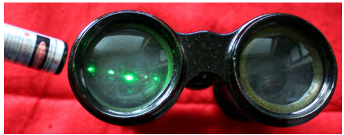
Figure 7 — Objective end of the Potter field glasses, with reflections from a 532-nm laser showing the boundaries of the contact crown and flint elements. Photograph by R.A. Rosenfeld.
