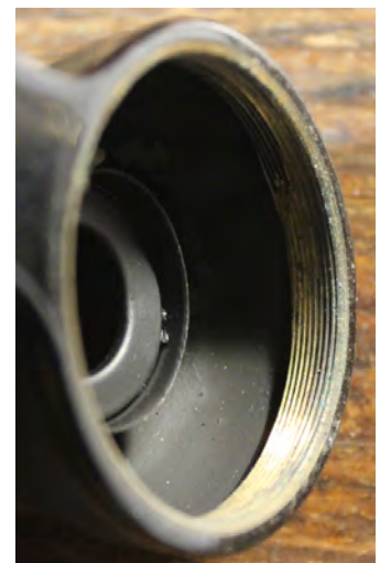
Figure 9 — Objective barrel of the Potter field glasses with objective cell removed, showing internal blackening, and field stop. Photograph by R.A. Rosenfeld.
