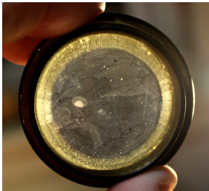
Figure 11 — Right-hand objective cell & doublet of the Potter field glasses showing balsam degradation around the edge. Photograph by R.A. Rosenfeld.
