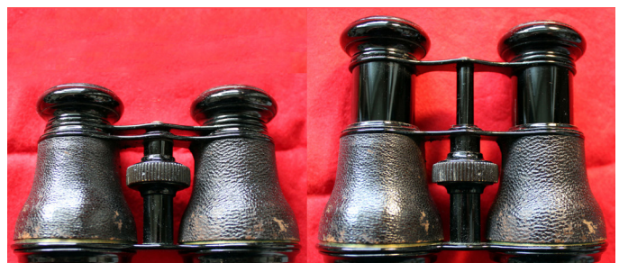
Figure 10 — The Potter field glasses with the eyepieces fully racked in (left), and fully racked out (right). Photograph by R.A. Rosenfeld.
