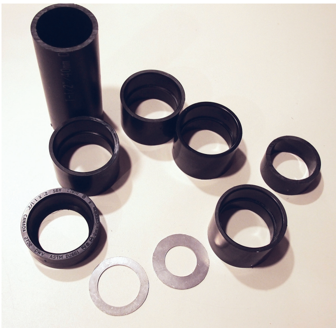
Figure 3 — ABS plastic components of the telescope baffles.
