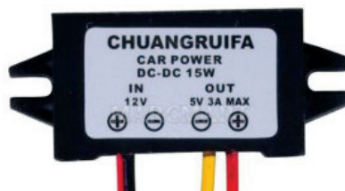
Figure 3 — 5V power for a USB hub, via purple lights for a Honda.
