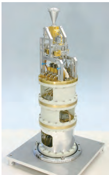
Figure 2 — The nucleus of the Band 3 receiver is a superconductor-insulator-superconductor (SIS) tunnel diode mixer, which down-converts the radio frequency (RF) signal collected by the radio telescope to an intermediate frequency (IF) signal centered at 8 GHz with a bandwidth of 8 GHz. The SIS detector must operate at a temperature of 4° Kelvin. A cryogenic high-electron-mobility transistor amplifier is used to amplify the IF signal by 40 dB before it is delivered to the ALMA Back-End System. Further details can be found at www.hia-ihh.nrc-cnrc.gc.ca/atrgv/alma_e.html .
