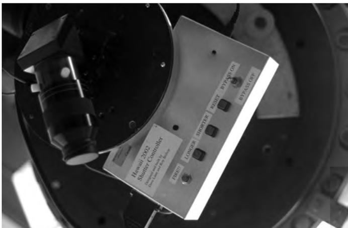
Figure 2 — A view of the lower end of the 0.61-m telescope. The shutter control circuit is in the rectangular box upon which are mounted the five switches that were used to adjust and activate the shutter. The 35-mm eyepiece is near the left side. (Photo by Roy Bishop)
