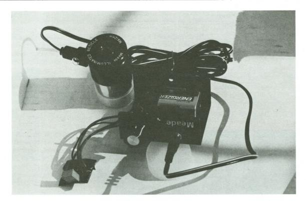
A photograph of the finished product. The additional circuitry that causes the blinking of the reticle is located on the small square circuit board in the lower left corner. The rest of the apparatus is a commercially produced illuminated reticle.
