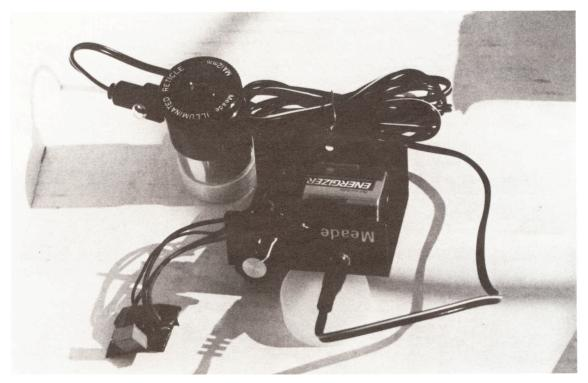
A photograph of the finished product. The additional circuitry that causes the blinking of the reticle is located on the small square circuit board in the lower left corner. The rest of the apparatus is a commercially produced illuminated reticle.
