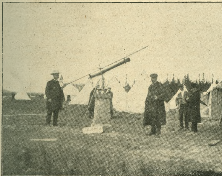
REV. I. J. KAVANAGH, S.J., AND HIS UNIQUE DEVICE FOR EXAMINATION OF THE OUTER CORONA AND STREAMERS.
