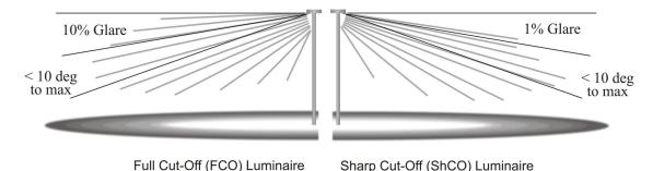
Figure 3.10.2 Comparison of FCO and ShCO shielding. FCO shielding permits 10% of the total emitted light to shine within 10-degrees below the horizon. ShCO shielding reduces this to only 1% and significantly reduces this glare.
