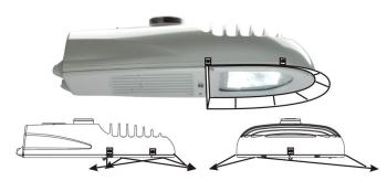
Figure 3.10.3 Sketch of luminaire shield. This is a sketch of what a shield could look like. The shape is based on earlier shields that were used on non cut-off cobra lights. The front and back surfaces should be designed to limit light trespass. Similar concepts should be used for other types of luminaires.
