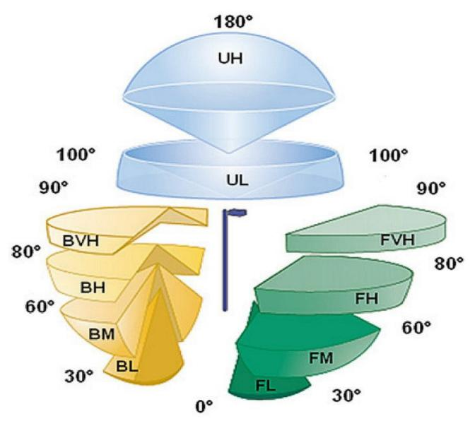
FCO luminaire preclude any up light (UH and UL = 0% of total emitted light). To minimize glare and light trespass that increases the impact area of the illumination should have BVH and FVH as close to 0% as possible. FCO fixtures allow 10% of the total light to be emitted in the zone from  $80^\circ$  to  $90^\circ$  of nadir (Glare Zone). However the preferred Sharp Cut-off designation only permits 1% in the Glare Zone, which can be achieved with FCO using and additive shield.
