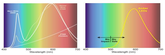
Figure 3.8 Spectra of Common Lamps
