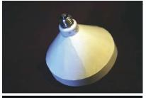
This example is made from cardboard with a coat of outdoor paint to protect it against weather. The exterior colour may be selected for it to blend in with the surroundings, the interior colour may be white to maximize the illumination, or black to reduce the brightness of the ground. If metal is used, care must be taken to prevent touching the electrical contacts at the bottom of the bulb.
