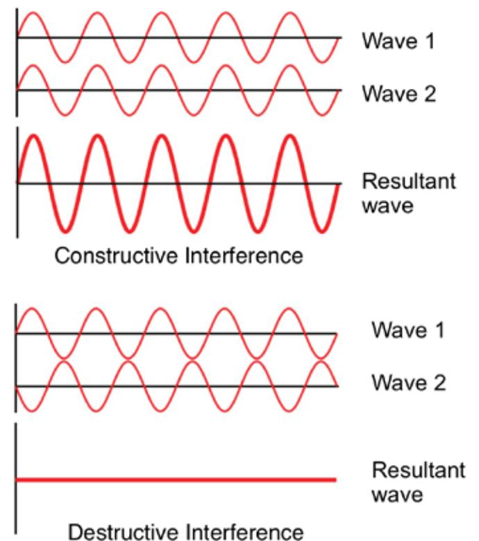
Figure 18 – Examples of constructive and destructive interference (graphic adapted from a Creative Commons source [29]).
