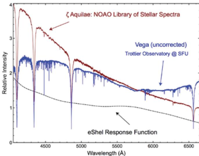
Figure 6 — Spectrum of Vega without correction for the overall response of the *eShel*/CCD chip, compared with a standardized spectrum of a star of the same spectral type. The dashed line is the computed response function of the spectrometer.
