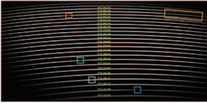
Figure 4 — *eShel* acquisition image for Vega. The yellow text identifies the central wavelength in each of the displayed orders. The coloured boxes identify some significant spectral features, as detailed in the text.
