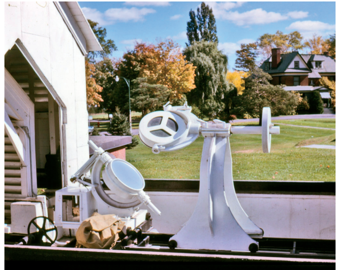
Figure 4 — Two plane mirrors of the three-mirror horizontal solar telescope, autumn 1963. The lower 24-inch mirror is mounted on an adjustable polar axis; it is the original coelostat purchased to observe the total solar eclipse of August 1905 in Labrador. The image-forming mirror is out of sight under the roll-back roof to the left. It reflects the beam, inclined slightly downward, to the right through a large opening in the casting that supports the upper plane mirror and toward a spectrometer housed in a basement laboratory. The Director’s House is in the background to the right.
