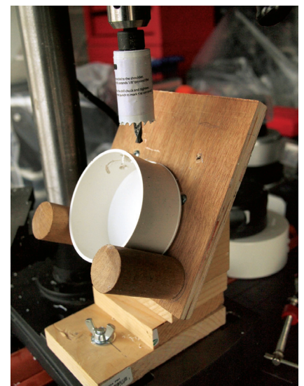
Figure 3 – The jig for drilling the hubs.
