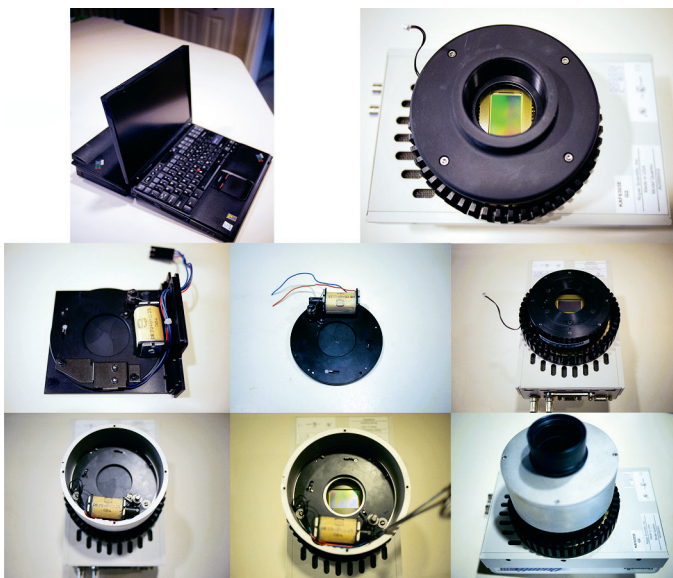
Figure 1 — Stages in the disassembly and reconstruction of the Quantix "astronomy-enabled" camera.
