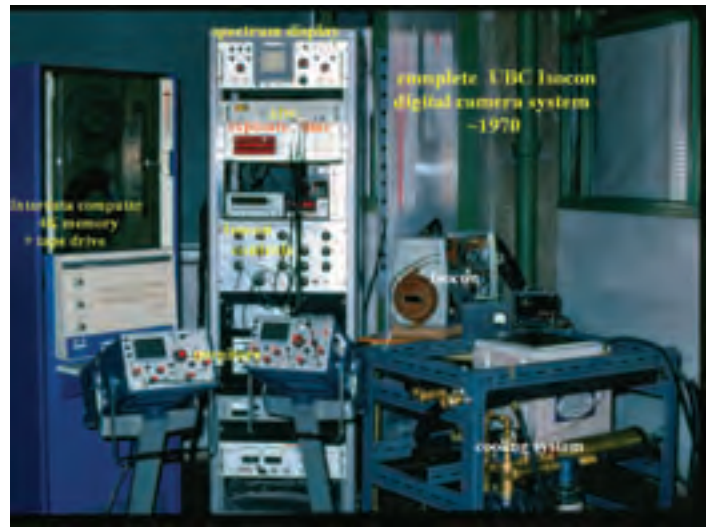
Figure 1 — The full Image Isocon digital camera system c 1970. The Isocon was a low-light-level version of a studio Orthocon having a 70-mm photocathode with magnetic scanning coils. It had 11 separate controls, many interactive! To avoid image spread during an integration, the tube was cooled to -10 °C by forced air circulating through a refrigerant. The Interdata computer had only 4K of memory and data were recorded on magnetic tape. The whole system had considerably less capability than the CCD camera in a modern cell phone.
