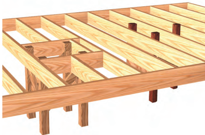
Figure 2 — Joists and framing. Use joist hangers and galvanized nails to frame the opening for the Dob base.
