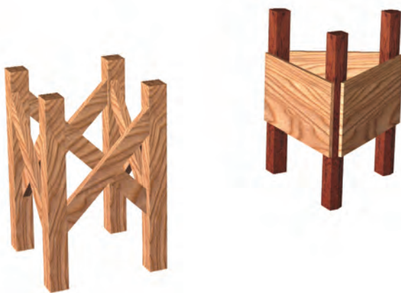
Figure 1 — Dob and tripod bases. Both the Dob base and the tripod base can be preassembled. Use braces to stiffen the assembly or, much easier, a plywood skirt.
