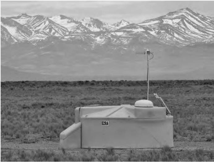
A view of surface detector “Ezra” on site in Argentina. One can see the battery box (left), the electronics dome (top), solar panels, and communications mast.
