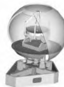
Figure 2. — A 1 to 100th scale wind-tunnel model of a large telescope dome. Image courtesy of NRC-HIA. For further details see the Web page at www.hia-aha.nrc-cnrc.gc.ca/main_e.html .
